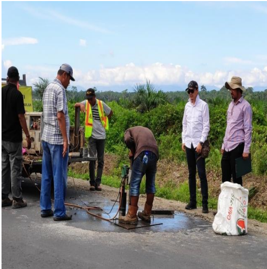
Gambar 41.. Pengambilan sample hotmix dan proses pengujian sample di laboratorium
